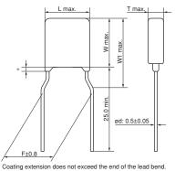
Coating extension does not exceed the end of the lead bend
