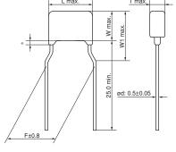
Coating extension does not exceed the end of the lead bend Lead Wire: Solder Coated CP Wire
