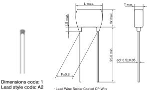
· Lead Wire: Solder Coated CP Wire
