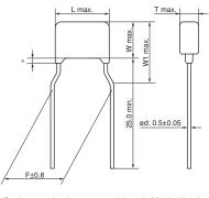
Coating extension does not exceed Lead Wire: Solder Coated CP Wire
