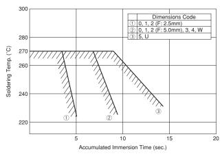
Perform soldering within tolerance range (shaded portion).
