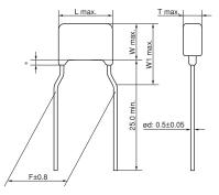
Coating extension does not exceed the end of the lead bend Lead Wire: Solder Coated CP Wire
