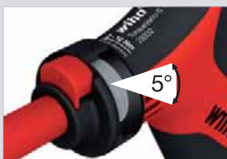
Finely toothed, switchable ratchet (72 teeth) with 5° switching angle.
