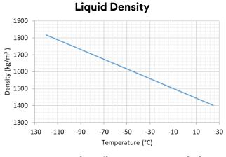
Liquid Density [kg/m<sup>3</sup>] = 1472.6 - 2.880 \* T[°C]
