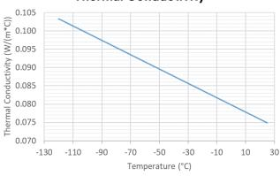
Thermal Conductivity [W·m<sup>-1</sup>·K<sup>-1</sup>] = 0.0798 - 0.000196 \* T[°C]
