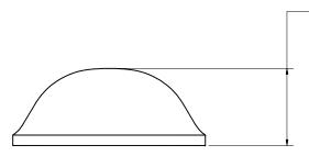
$-.150\pm.02$  in  $[3.81\pm0.51$  mm] THIS DIMENSION INCLUDES THE ADHESIVE. IT DOES NOT INCLUDE THE TAPE LINER.
