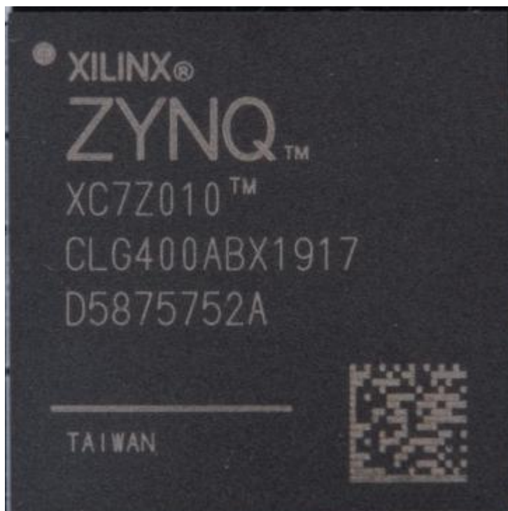
Figure 2-2-3: The XC7Z010 chip used on the Core Board
