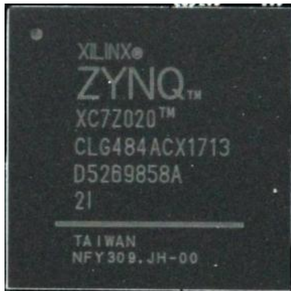
Figure 1-2-3: The XC7Z020 chip
