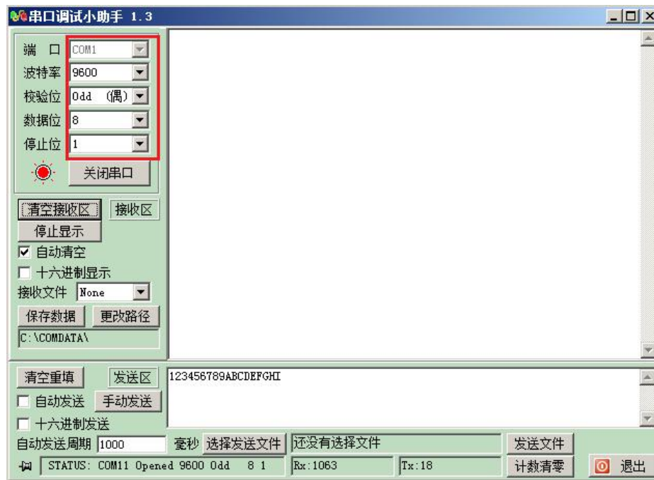
Figure 3-3: The Specific Configuration of Serial Debugging Assistant
