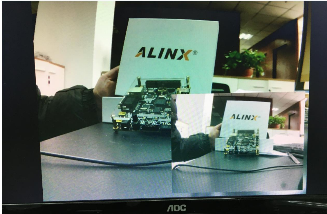
Figure 4-4: OV5642 Picture-in-picture Effect on the VGA Display
