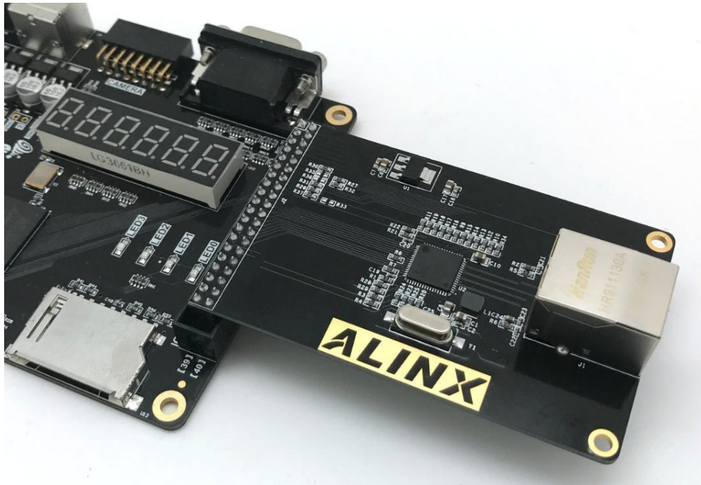
Figure 3-1: Hardware connection to AX301 FPGA Board and AN8211
