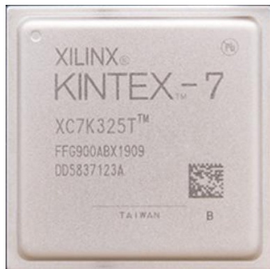
Figure 2.2-2: FPGA chip on board
