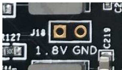
Figure 3-3: Test Points for Power supply on the Board
