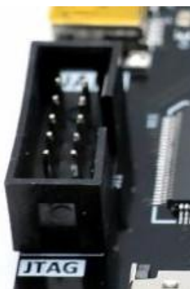
Figure 3-10-2: JTAG Interface on the Expansion Board
