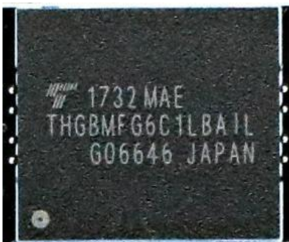
Figure 2-5-2: eMMC Flash on the Core Board
