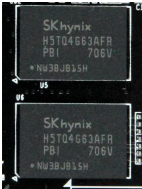
Figure 2-3-2: DDR3 DRAM on the Core Board
