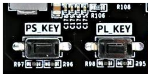
Figure 3-12-2: The User Button on the Expansion Board
