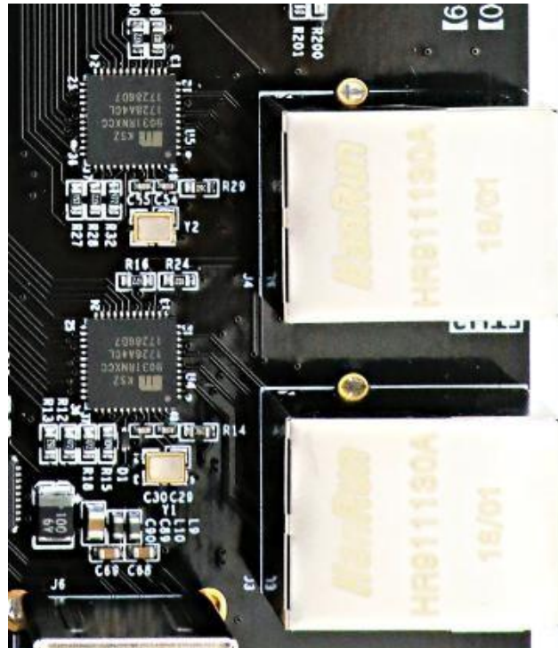
Figure 3-2-3: PS and PL Ethernet GPHY chips on Expansion Board
