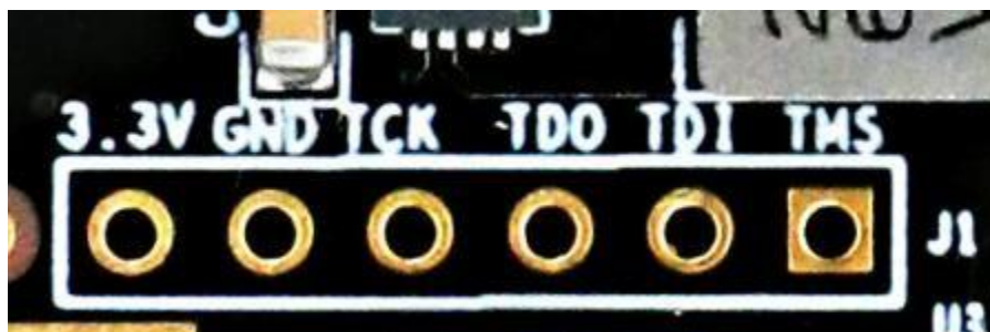
Figure 2-10-2: JTAG interface on the core board
