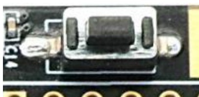
Figure 2-9-2: Reset button on the Core Board
