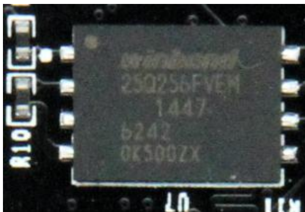
Figure 2-4-2: QSPI Flash on the Core Board
