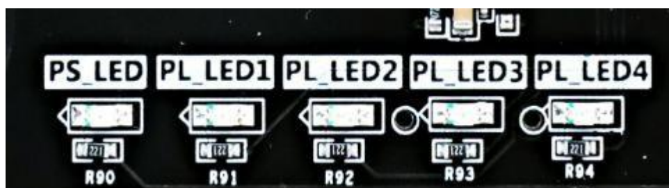
Figure 3-11-2: LEDs on the Expansion Board
