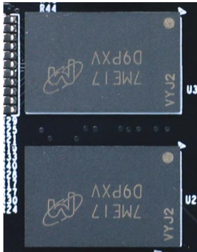
Figure 2-4-2: The DDR3 on the Core Board
