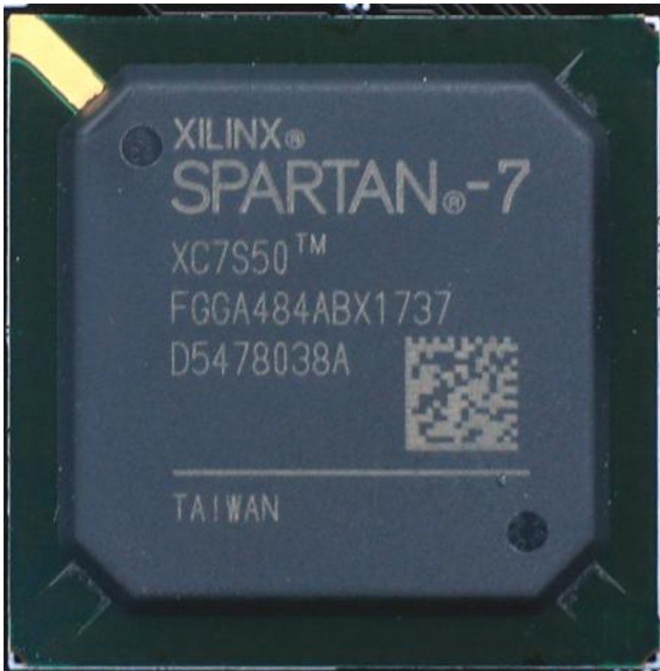
Figure 2-2-2: FPGA chip on board
