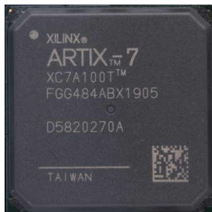
Figure 2-2-2: FPGA chip on board
