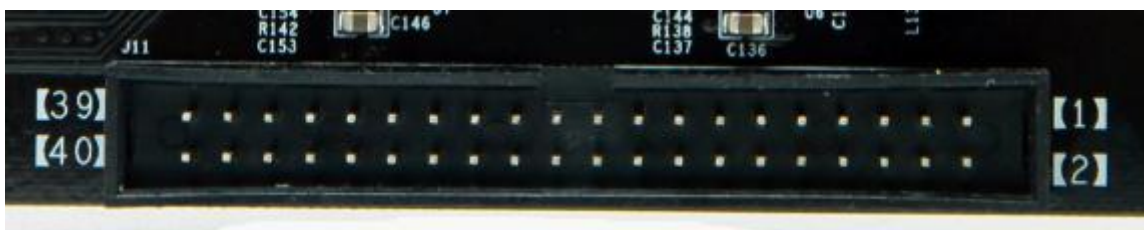
Figure 3-6-2: Expansion header J11 on the Carrier Board
