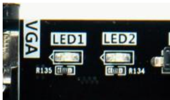
Figure 3-9-2: The User LEDs on the Carrier Board
