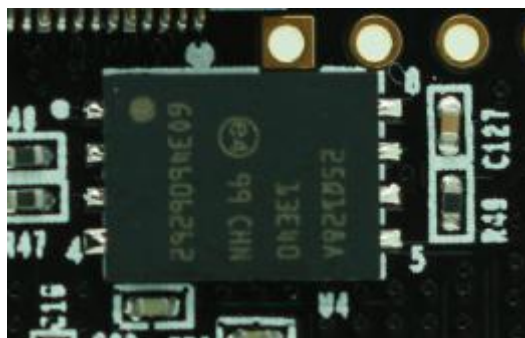
Figure 2-5-2: QSPI on the Core Board
