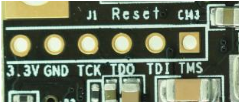
Figure 2-8-2: JTAG Interface on Core Board
