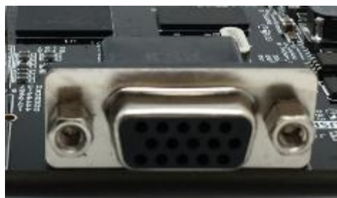
Figure 3-4-3: VGA Display Interface on the Carrier Board
