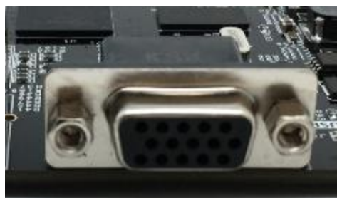
Figure 3-4-3: VGA Display Interface on the Carrier Board
