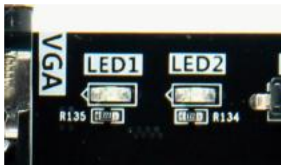
Figure 3-9-2: The User LEDs on the Carrier Board
