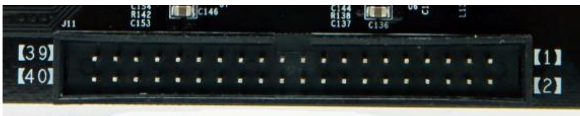
Figure 3-6-2: Expansion header J11 on the Carrier Board
