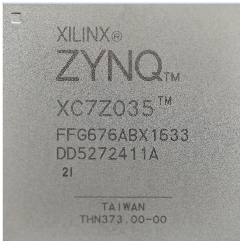
Figure 2-3: The XC7Z035 chip used on the Core Board
