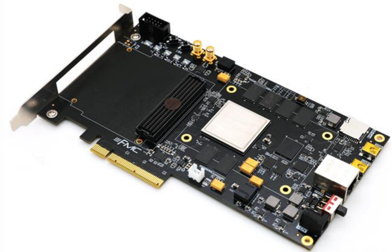
Figure 1: AX7450B development board
