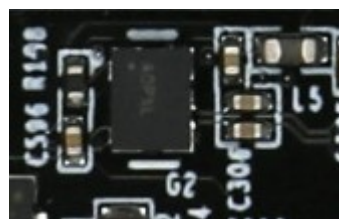
Figure 2-6-5: Programmable clock source on the board
