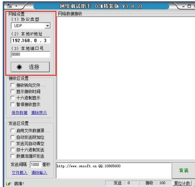
At this time, the network data receiving window will display the Ethernet packet "Hello ALINX HEIJIN" sent by the FPGA to the PC. The IP address of the target host must be consistent with the IP address in the FPGA program, and the target port number must be consistent with that in the FPGA program (8080). Network display as shown in the following figure:
