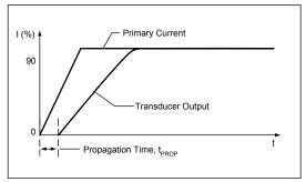
**Response time (t\_{RESPONSE}):** The time interval between a) when the primary current signal reaches 90% of its final value, and b) when the sensor reaches 90% of its output corresponding to the applied current.
