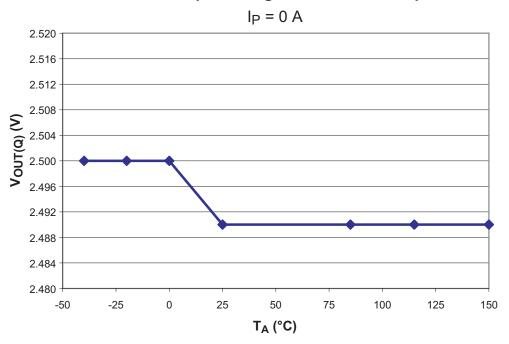
Zero Current Output Currrent versus Ambient Temperature
