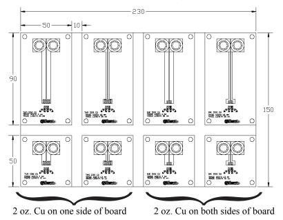
An ACS704 device was soldered onto each PC board before beginning the thermal testing. Thermal management tests were conducted with the following test conditions:
