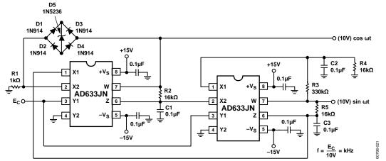
Figure 21. Voltage-Controlled Quadrature Oscillator
