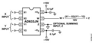
Figure 11. Basic Multiplier Connections
