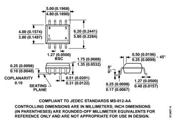
Figure 24. 8-Lead Standard Small Outline Package [SOIC\_N] Narrow Body (R-8)
