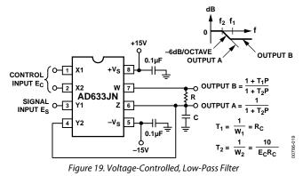
The voltage at Output B, the direct output of the AD633, has the same response up to frequency  $f_1$ , the natural breakpoint of RC filter, and then levels off to a constant attenuation of  $f_1/f_2 = E_C/10$ .
