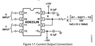
This arrangement forms the basis of voltage-controlled integrators and oscillators as is shown later in this section. The transfer function of this circuit has the form
