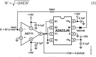
Figure 14. Connections for Square Rooting
