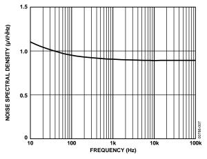
Figure 8. Noise Spectral Density vs. Frequency
