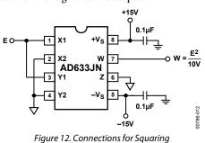
When the input is a sine wave E sin  $\omega$ t, this squarer behaves as a
