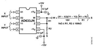
Figure 16. Connections for Variable Scale Factor
