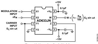
Figure 18. Linear Amplitude Modulator
