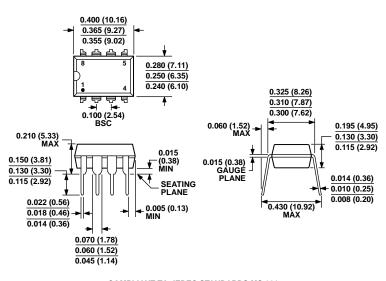
COMPLIANT TO JEDEC STANDARDS MS-001 CONTROLLING DIMENSIONS ARE IN INCHES; MILLIMETER DIMENSIONS (IN PARENTHESES) ARE ROUNDED-OFF INCH EQUIVALENTS FOR REFERENCE ONLY AND ARE NOT APPROPRIATE FOR USE IN DESIGN. CORNER LEADS MAY BE CONFIGURED AS WHOLE OR HALF LEADS.
