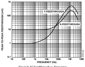
Figure 9. AC Feedthrough vs. Frequency
