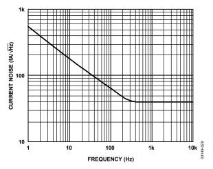
Figure 29. Current Noise Spectral Density vs. Frequency
