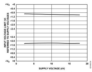
Figure 19. Input Voltage Limit vs. Supply Voltage, G = 1
