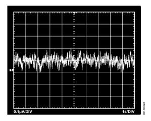
Figure 28. 0.1 Hz to 10 Hz RTI Voltage Noise (G = 1000)
