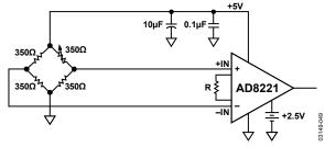
Figure 49. Precision Strain Gage
