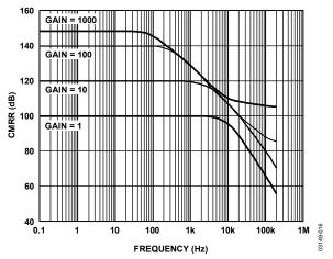
Figure 16. CMRR vs. Frequency, RTI
