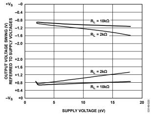
Figure 20. Output Voltage Swing vs. Supply Voltage, G = 1
