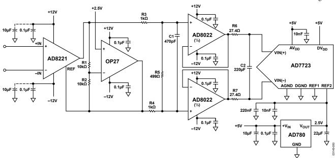
Figure 50. Interfacing to a Differential Input ADC
