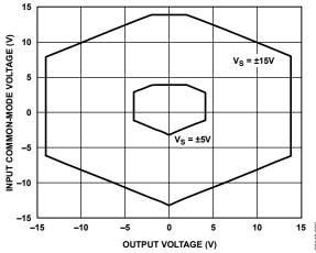
Figure 8. Input Common-Mode Range vs. Output Voltage, G = 100
