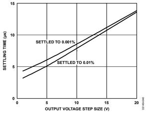
Figure 40. Settling Time vs. Step Size (G = 1)
