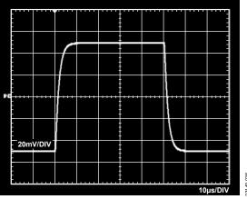
Figure 38. Small Signal Response, G = 100,  $R_L = 2 k\Omega$ ,  $C_L = 100 pF$
