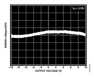
Figure 25. Gain Nonlinearity, G = 1000,  $R_L = 10 \text{ k}\Omega$
