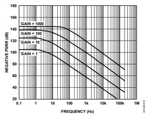
Figure 13. Negative PSRR vs. Frequency, RTI (G = 1 to 1000)
