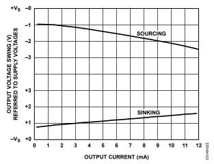
Figure 22. Output Voltage Swing vs. Output Current, G = 1
