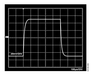
Figure 39. Small Signal Response, G = 1000,  $R_L = 2 k\Omega$ ,  $C_L = 100 pF$
