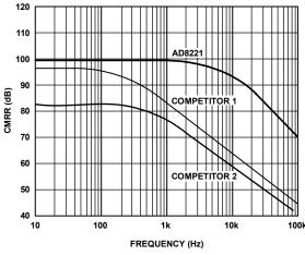
Figure 2. Typical CMRR vs. Frequency for G = 1
