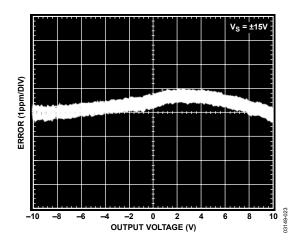
Figure 23. Gain Nonlinearity, G = 1,  $R_L = 10 \text{ k}\Omega$
