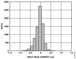
Figure 5. Typical Distribution of Input Bias Current
