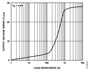
Figure 21. Output Voltage Swing vs. Load Resistance
