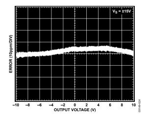
Figure 24. Gain Nonlinearity, G = 100,  $R_L = 10 \text{ k}\Omega$
