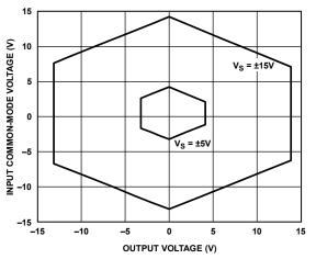
Figure 7. Input Common-Mode Range vs. Output Voltage, G = 1
