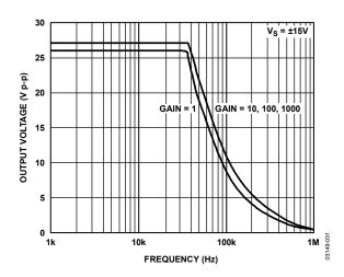
Figure 31. Large Signal Frequency Response
