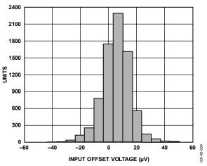
Figure 4. Typical Distribution of Input Offset Voltage
