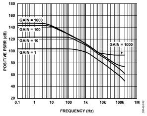
Figure 12. Positive PSRR vs. Frequency, RTI (G = 1 to 1000)
