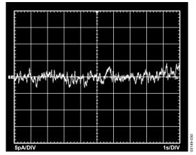
Figure 30. 0.1 Hz to 10 Hz Current Noise
