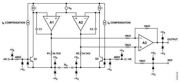
Figure 42. Simplified Schematic
