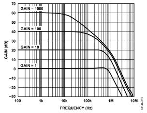
Figure 15. Gain vs. Frequency
