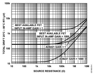
Figure 14. Total Drift vs. Source Resistance
