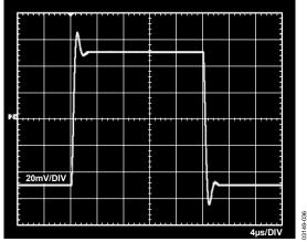
Figure 36. Small Signal Response, G = 1,  $R_L = 2 k\Omega$ ,  $C_L = 100 pF$
