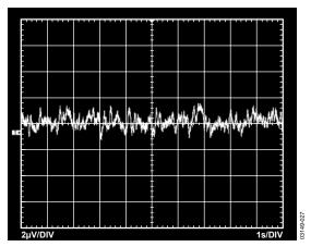
Figure 27. 0.1 Hz to 10 Hz RTI Voltage Noise (G = 1)
