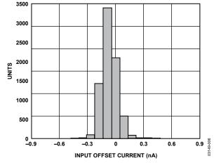
Figure 6. Typical Distribution of Input Offset Current
