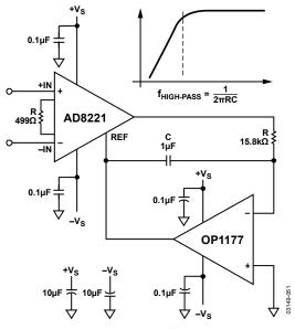
Figure 51. AC-Coupled Circuit
