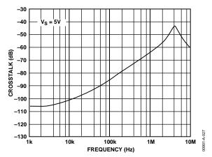
Figure 27. Crosstalk vs. Frequency
