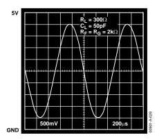
Figure 29. Output Swing,  $V_5 = 5 V$ , G = -1
