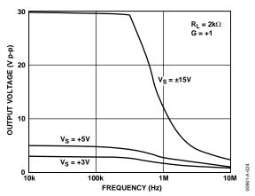
Figure 24. Large Signal Frequency Response
