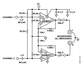
Figure 42. 3 V Single-Supply Stereo Headphone Driver
