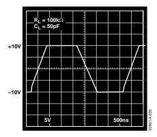
Figure 35. Pulse Response,  $V_S = \pm 15 \text{ V}$ , G = +1
