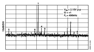
Figure 41. FFT of AD1672 Output Driven by AD823
