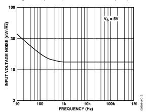
Figure 16. Input Voltage Noise vs. Frequency
