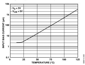
Figure 9. Input Bias Current vs. Temperature
