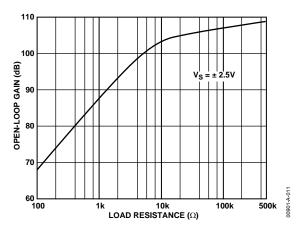
Figure 11. Open-Loop Gain vs. Load Resistance
