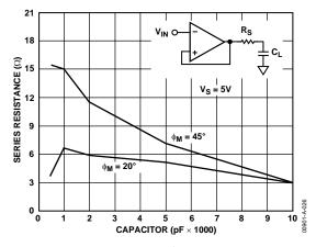
Figure 26. Capacitive Load vs. Series Resistance
