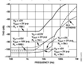
Figure 13. Total Harmonic Distortion vs. Frequency
