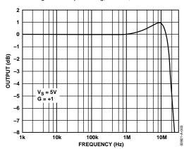
Figure 3. Small Signal Bandwidth, G = +1
