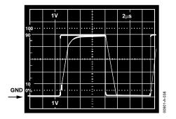
Figure 38. AD823 Input Response: Response with  $R_P = 0$ ,  $V_{IN}$  from 0 to  $V_S$
