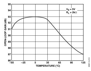
Figure 14. Open-Loop Gain vs. Temperature
