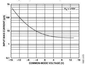
Figure 10. Input Bias Current vs. Common-Mode Voltage
