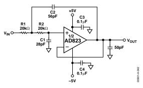
Figure 43. Second-Order Low-Pass Filter
