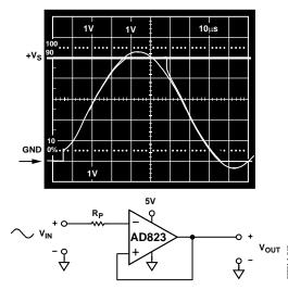
Figure 39. AD823 Input Response:  $V_{IN} = 0 \text{ to } +V_S + 200 \text{ mV}, V_{OUT} = 0 \text{ to } +V_S, R_P = 49.9 \text{ k}\Omega$
