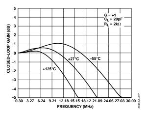
Figure 17. Closed-Loop Gain vs. Frequency
