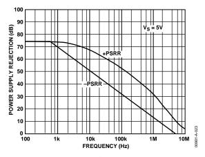
Figure 23. Power Supply Rejection vs. Frequency
