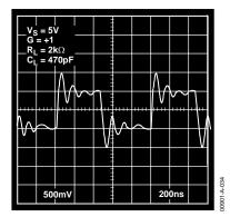
Figure 34. Pulse Response,  $V_S = 5 V$ , G = +1,  $C_L = 470 pF$
