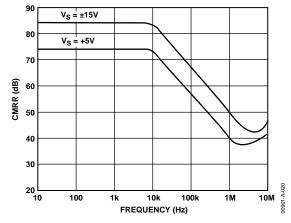
Figure 20. Common-Mode Rejection vs. Frequency
