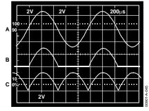
Figure 46. Single-Supply Half-Wave and Full-Wave Rectifier
