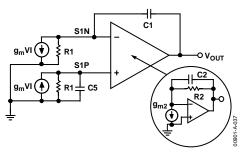
Figure 37. Small Signal Schematic
