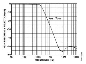
Figure 44. Frequency Response of Filter
