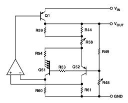
Figure 1. Simplified Schematic
