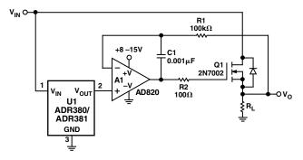
Figure 5. ADR380/ADR381 for Precision High Current Voltage Source
