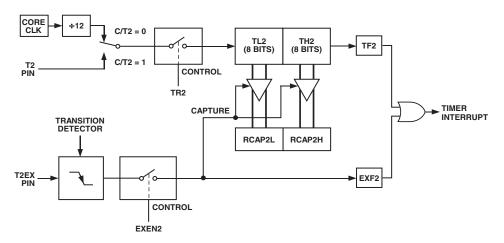
Figure 31. Timer/Counter 2, 16-Bit Capture Mode
