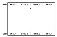
Figure 16. User Flash/EE Memory Configuration
