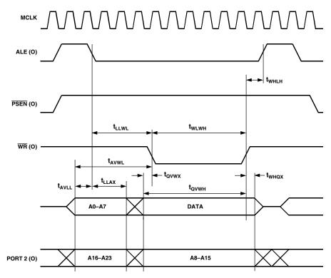
Figure 53. External Data Memory Write Cycle
