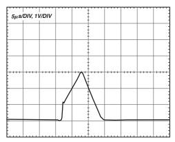
Figure 24. DAC Output Spike at DAC Enable
