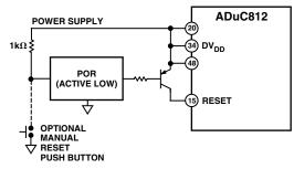
Figure 42. External Active Low POR Circuit
