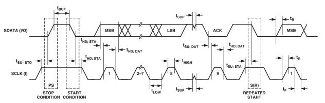
Figure 55. I<sup>2</sup>C Compatible Interface Timing
