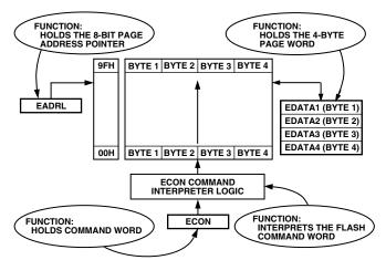
Figure 17. User Flash/EE Memory Control and Configuration
