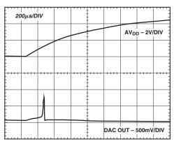
Figure 23. DAC Output Spike at Chip Power-Up
