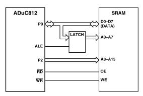
Figure 38. External Data Memory Interface (64K Address Space)
