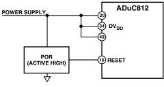
Figure 41. External Active High POR Circuit
