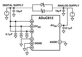
Figure 43. External Dual-Supply Connections
