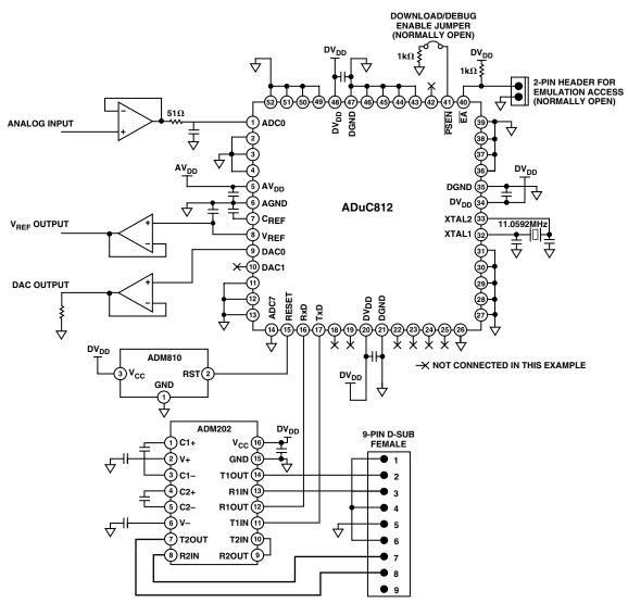
Figure 46. Typical System Configuration
