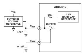
Figure 10. Using an External Voltage Reference
