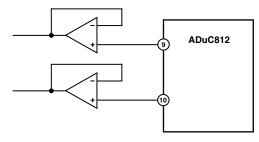
Figure 22. Buffering the DAC Outputs
