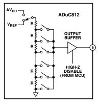
Figure 18. Resistor String DAC Functional Equivalent
