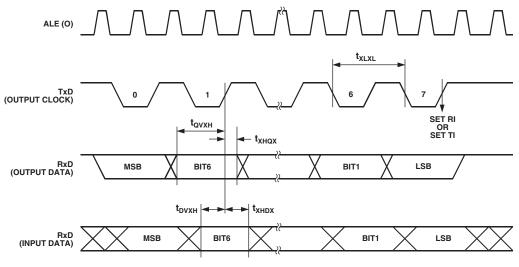
Figure 54. UART Timing in Shift Register Mode
