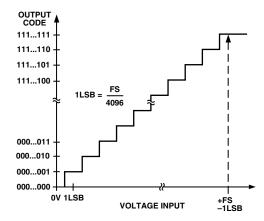
Figure 5. ADC Transfer Function
