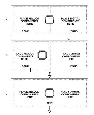
Figure 45. System Grounding Schemes
