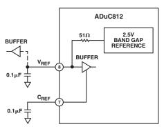
Figure 9. Decoupling  $V_{REF}$  and  $C_{REF}$
