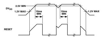
Figure 40. External POR Timing
