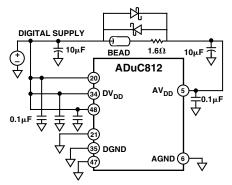
Figure 44. External Single-Supply Connections
