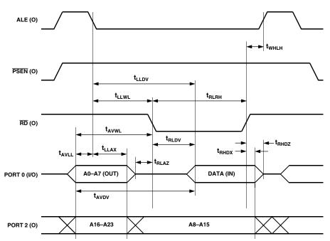
Figure 52. External Data Memory Read Cycle
