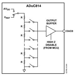
Figure 38. Resistor String DAC Functional Equivalent
