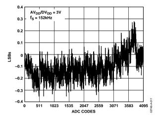
Figure 4. Typical INL Error,  $V_{DD} = 3 V$
