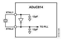
Figure 54. External Parallel Resonant Crystal Connections
