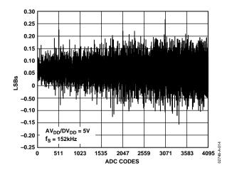
Figure 7. Typical DNL Error,  $V_{DD} = 5 V$
