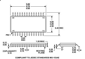
Figure 67. 28-Lead Thin Shrink Small Outline Package (TSSOP) (RU-28)
