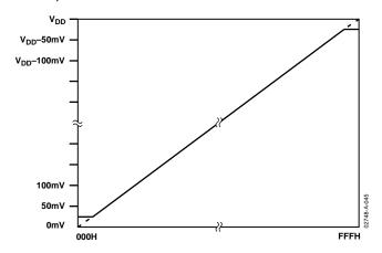
Figure 39. Endpoint Nonlinearities Due to Amplifier Saturation
