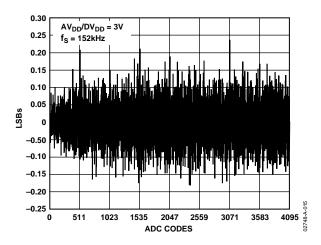
Figure 8. Typical DNL Error,  $V_{DD} = 3 V$
