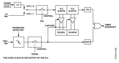
Figure 50. Timer/Counter 2, 16-Bit Capture Mode
