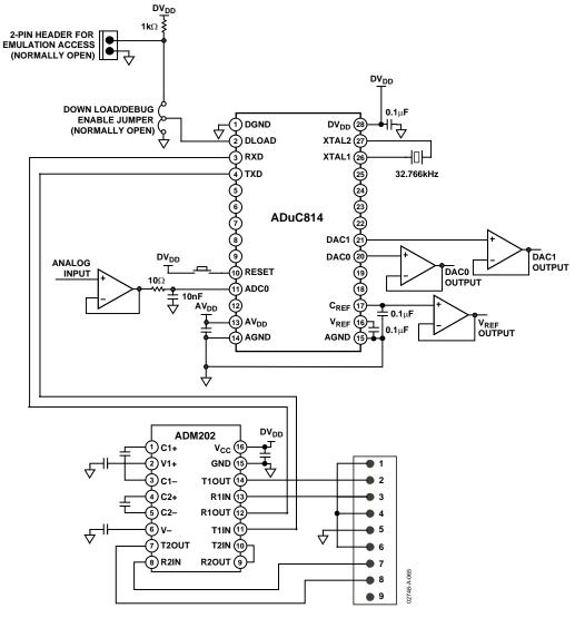
Figure 59. Typical ADuC814 System Connection Diagram
