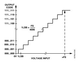
Figure 23. ADuC814 ADC Transfer Function
