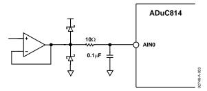
Figure 26. Buffering Analog Inputs
