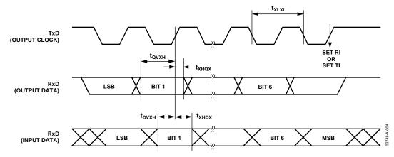
Figure 62. UART Timing in Shift Register Mode
