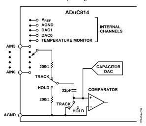
Figure 25. Internal ADC Structure
