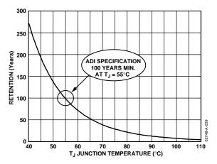
Figure 33. Flash/EE Memory Data Retention
