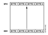
Figure 36. Flash/EE Data Memory Configuration
