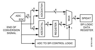
Figure 31. High Speed Data Capture Logic
