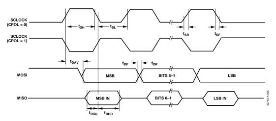
Figure 63. SPI Master Mode Timing (CPHA = 1)
