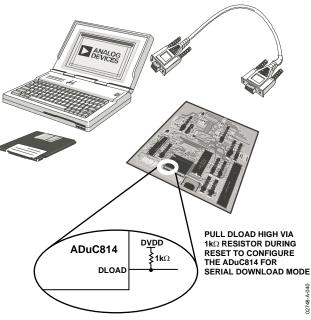
Figure 34. Flash/EE Memory Serial Download Mode Programming
