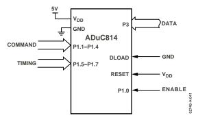
Figure 35. Flash/EE Memory Parallel Programming
