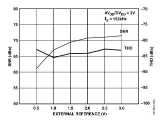
Figure 16. Typical Dynamic Performance vs.  $V_{REF}$ ,  $V_{DD} = 3 V$
