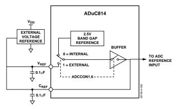
Figure 28. Using an External Voltage Reference
