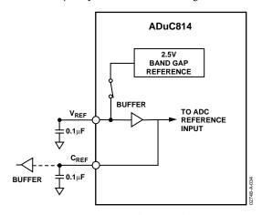
Figure 27. Decoupling VREF and CREF
