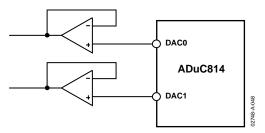
Figure 42. Buffering the DAC Outputs
