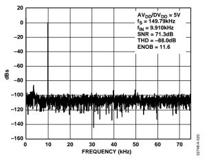
Figure 13. ADuC814 Dynamic Performance at  $V_{DD} = 5 V$
