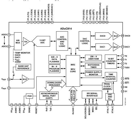
Figure 17. ADuC814 Block Diagram
