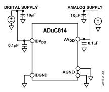
Figure 55. External Dual-Supply Connections
