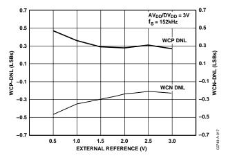
Figure 10. Typical Worst-Case DNL Error vs.  $V_{REF}$ ,  $V_{DD} = 3 V$
