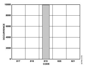
Figure 11. Code Histogram plot,  $V_{DD} = 5 V$
