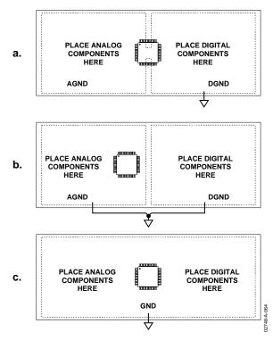
Figure 58. System Grounding Schemes
