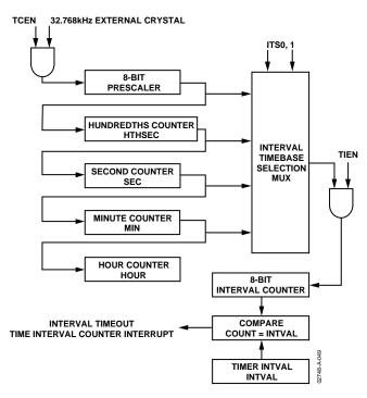
Figure 43. Time Interval Counter, Simplified Block Diagram
