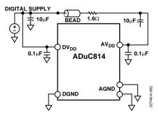
Figure 56. External Single-Supply Connections
