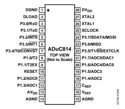
Figure 2. Pin Configuration
