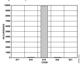
Figure 12. Code Histogram Plot,  $V_{DD} = 3 V$
