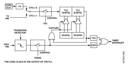
Figure 49. Timer/Counter 2, 16-Bit Autoreload Mode
