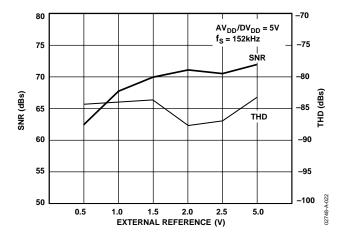
Figure 15. Typical Dynamic Performance vs.  $V_{REF}$ ,  $V_{DD} = 5 V$
