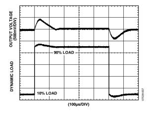
Figure 8. Typical V<sub>ISO</sub> Transient Load Response, 5 V Output, 10% to 90% Load Step
