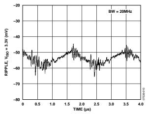
Figure 11. Typical V<sub>ISO</sub> = 3.3 V, Output Voltage Ripple at 90% Load
