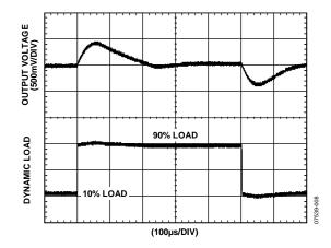
Figure 9. Typical V<sub>ISO</sub> Transient Load Response, 3 V Output, 10% to 90% Load Step
