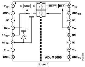
*iso*Power uses high frequency switching elements to transfer power through its transformer. Special care must be taken during printed circuit board (PCB) layout to meet emissions standards. See the AN-0971 Application Note for board layout recommendations.
