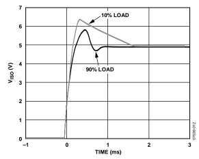
Figure 12. Typical  $V_{ISO} = 5 V$ , Output Voltage Startup Transient at 10% and 90% Load
