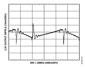
Figure 16. Typical V<sub>ISO</sub> = 3.3 V Output Voltage Ripple at 90% Load
