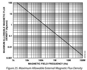
For example, at a magnetic field frequency of 1 MHz, the maximum allowable magnetic field of 0.2 kgauss induces a voltage of 0.25 V at the receiving coil. This voltage is approximately 50% of the sensing threshold and does not cause a faulty output transition. Similarly, if such an event occurs during a transmitted pulse (and is of the worst-case polarity), it reduces the received pulse from >1.0 V to 0.75 V, which is still well above the 0.5 V sensing threshold of the decoder.
