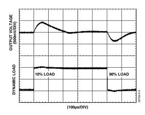
Figure 14. Typical V  $_{\rm ISO}$  Transient Load Response, 3.3 V Output, 10% to 90% Load Step
