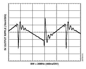
Figure 15. Typical V<sub>ISO</sub> = 5 V Output Voltage Ripple at 90% Load
