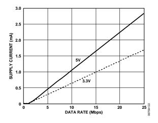
Figure 22. Typical I<sub>ISO (D)</sub> Dynamic Supply Current per Output (15 pF Output Load)
