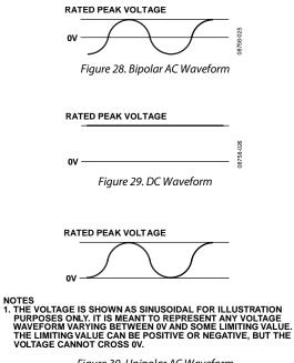
Figure 30. Unipolar AC Waveform
