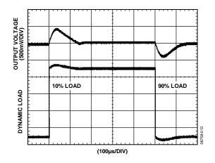
Figure 13. Typical V<sub>ISO</sub> Transient Load Response, 5 V Output, 10% to 90% Load Step
