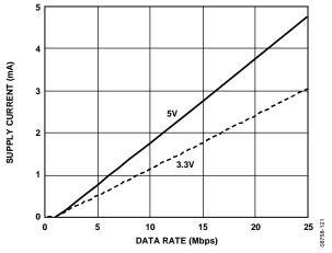
Figure 21. Typical I<sub>ISO (D)</sub> Dynamic Supply Current per Input
