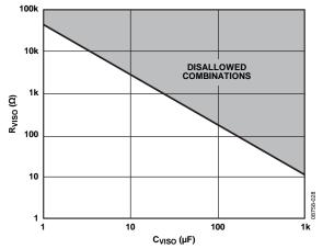
Figure 31. Maximum Capacitive Load for Proper Restart
