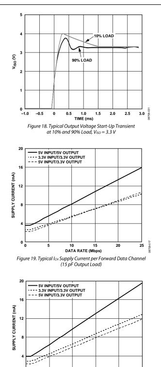
758-120 5 15 20 25 0 10 DATA RATE (Mbps) Figure 20. Typical I<sub>CH</sub> Supply Current per Reverse Data Channel (15 pF Output Load)
