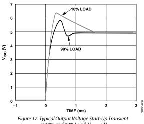
at 10% and 90% Load,  $V_{ISO} = 5 V$
