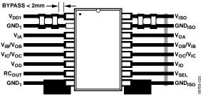
Figure 23. Recommended Printed Circuit Board Layout
