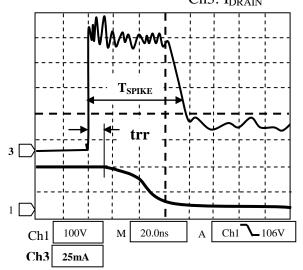
**Figure 4.** Switch-On-Off Transition. Ch1: V<sub>DRAIN</sub>, Ch3: I<sub>DRAIN</sub>
