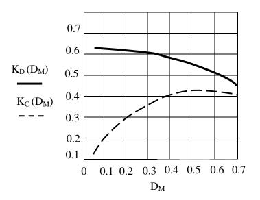
Fig.1. Conduction Loss Coefficients  $K_{C}$  and  $K_{D}$  EMI Filter
