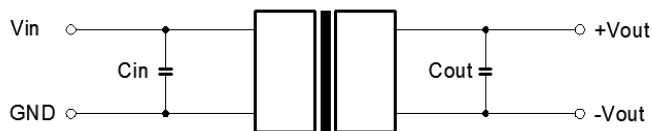
Figure 1. Typical external circuit
