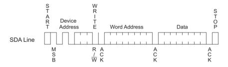
Page Write: The 16K EEPROM devices are capable of a 16-byte Page Write.
