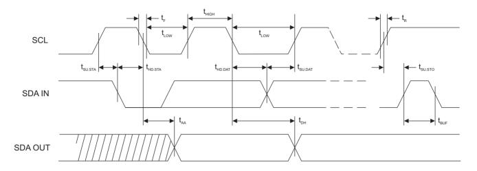
Figure 6-6. Write Cycle Timing
