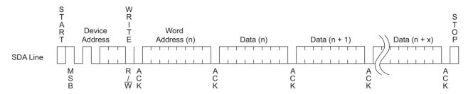
**Acknowledge Polling:** Once the internally timed write cycle has started and the EEPROM inputs are disabled, Acknowledge Polling can be initiated. This involves sending a Start Condition followed by the device address word. The Read/Write bit is representative of the operation desired. Only if the internal write cycle has completed will the EEPROM respond with a zero allowing the Read or Write sequence to continue.
