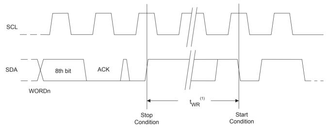
Note: 1. The write cycle time t<sub>WR</sub> is the time from a valid Stop Condition of a Write sequence to the end of the internal clear/write cycle.
