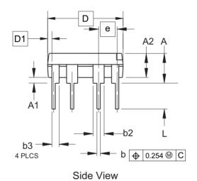
COMMON DIMENSIONS (Unit of Measure = mm)
