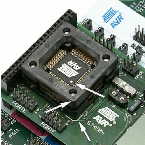
Figure 3-3: Placing the AVR in the ZIF socket
