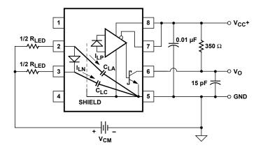
Figure 13. Recommended drive circuit for High-CMR.
