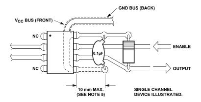
Figure 11. Recommended printed circuit board layout.
