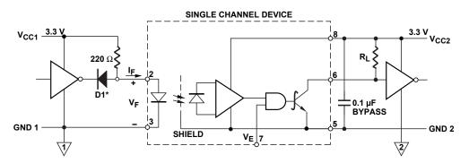
\*DIODE D1 (1N916 OR EQUIVALENT) IS NOT REQUIRED FOR UNITS WITH OPEN COLLECTOR OUTPUT.
