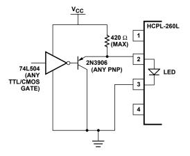
Figure 15. TTL interface circuit.
