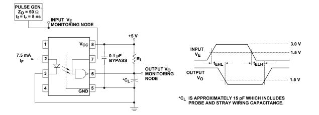
Figure 9. Test circuit for t<sub>EHL</sub> and t<sub>ELH</sub>.
