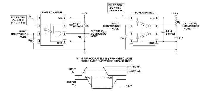
Figure 6. Test circuit for t<sub>PHL</sub> and t<sub>PLH</sub>.
