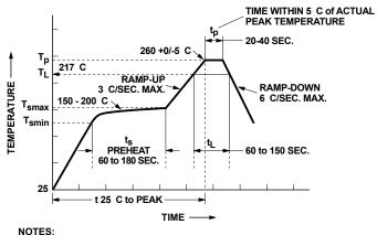
THE TIME FROM 25 C to PEAK TEMPERATURE = 8 MINUTES MAX.  $T_{smax}$  = 200 C,  $T_{smin}$  = 150 C
