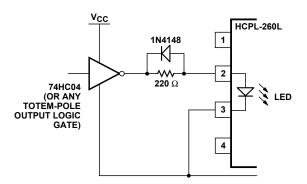
Figure 17. CMOS gate drive circuit.
