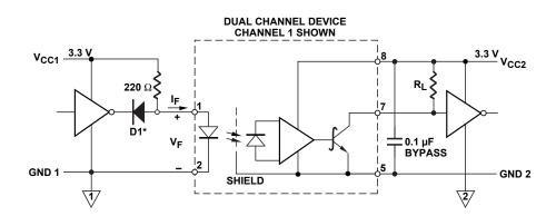
Figure 12. Recommended LVTTL interface circuit.
