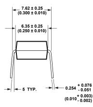
DIMENSIONS IN MILLIMETERS AND (INCHES). \* MARKING CODE LETTER FOR OPTION NUMBERS "V" = OPTION 060 OPTION NUMBER 500 NOT MARKED.
