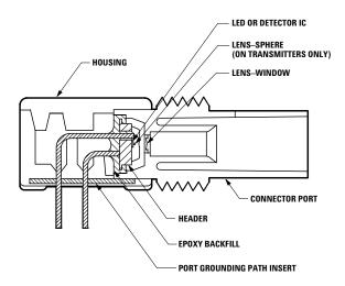
Figure 1. HFBR-0400Z ST Series Cross-Sectional View.
