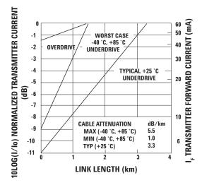
Figure 4. HFBR-14x2Z/HFBR-24x2Z Link Design Limits with 100/140 μm Cable.
