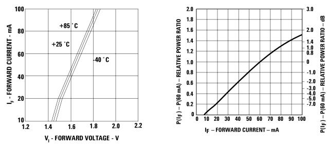
Figure 9. Forward Voltage and Current Characteristics.
