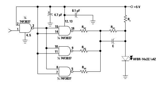
Figure 11. Recommended Drive Circuit.
