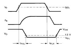
Figure 19. Propagation delay test waveforms.
