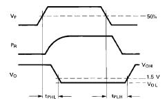
$\label{lem:Figure 26.Propagation delay test waveforms.}$
