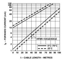
Figure 21. Guaranteed system performance with standard cable.
