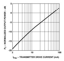
Figure 10. Normalized typical output power vs. drive current.
