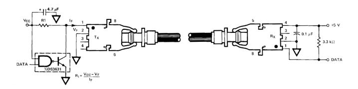
Figure 20. Typical 40 kBd interface circuit.
