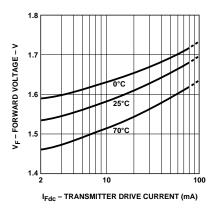
Figure 9. Typical forward voltage vs. drive current.
