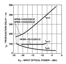
Figure 8. Typical link propagation delay vs. optical power.
