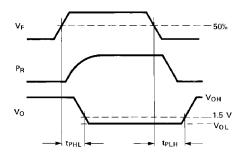
Figure 6. Propagation delay test waveforms.
