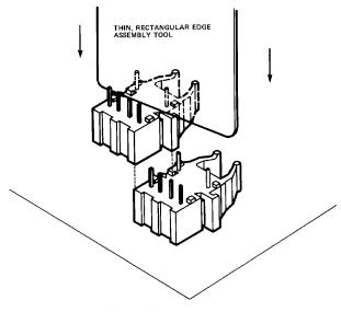
Figure 1. Interlocked (stacked) horizontal or vertical packages.
