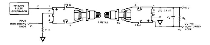
Figure 23. 40 kBd propagation delay test circuit.
