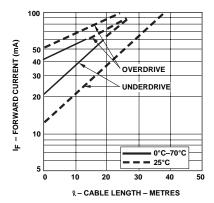
Figure 3. Guaranteed system performance with standard cable (HFBR-15X1Z/25X1Z).
