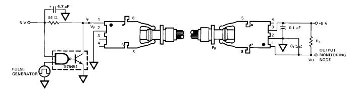
Figure 5. 5 MBd propagation delay test circuit.
