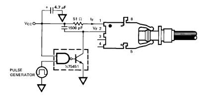
Figure 16. 1 MBd propagation delay test circuit.
