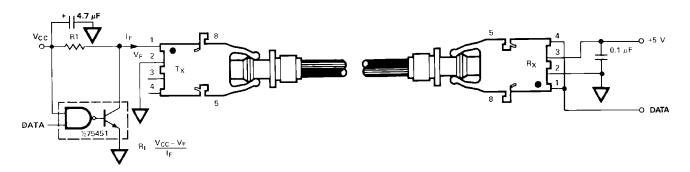
Figure 2. Typical 5 MBd interface circuit.
