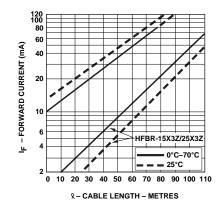
Figure 22. Guaranteed system performance with improved cable.
