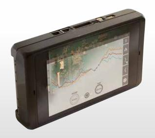
With back-printed glass plate, bonded touch screen / display unit + SBC.
