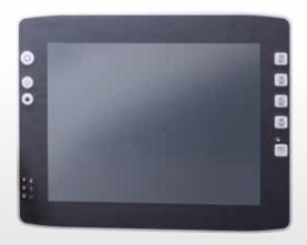
**Customised supporting plate**Resistive touch screen combined with customised membrane keypad.
