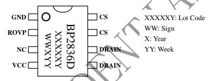
Figure 2. Pin configuration
