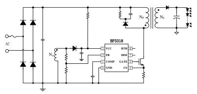
Figure 1. Typical application circuit for BP3318
