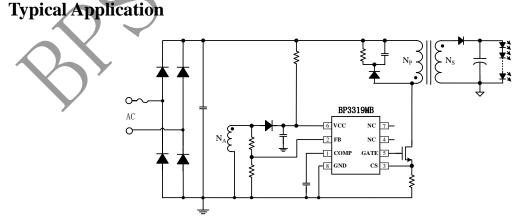
Figure 1. Typical application circuit for BP3319MB
