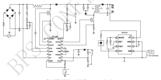
Fig.2 BP3368 for 1-10V Dimming Application
