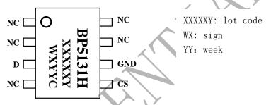
Fig 2 BP5131HC Pin Mapping
