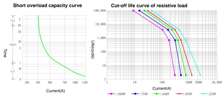
Note: Except for special note, the ambient temperature of electrical durability test is 23  $^{\circ}$ C, and the on-break ratio is: 1s: 9s
