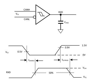
Figure 8-2 Receiver Test Circuit and Measurement
