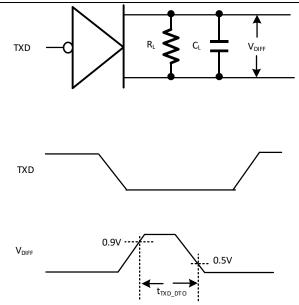
Figure 8-5 Transmitting Dominant Timeout Timing Diagram
