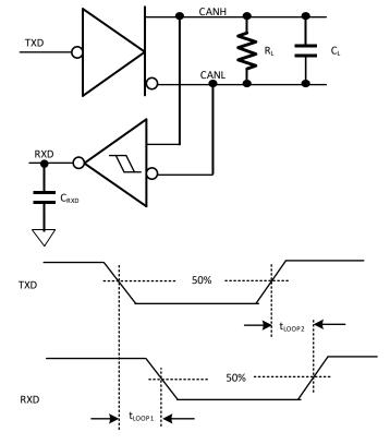
Figure 8-3 TXD to RXD Loop Delay
