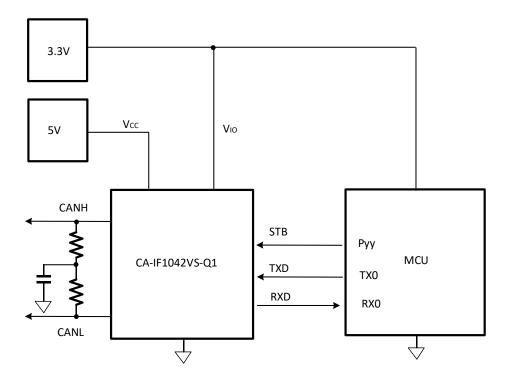
Figure 10-2 Typical Application Circuit for the CA-IF1042VS-Q1
