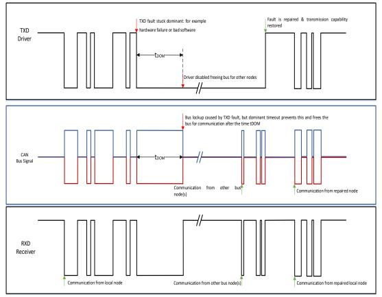
Figure 9-3 Transmitter-Dominant Timeout Protection
