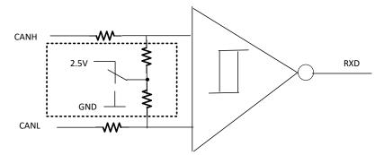
Figure. 9-2 Receiver Input/Transmitter Output Bias Circuit
