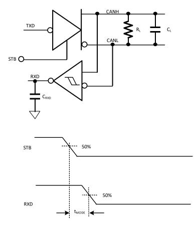
Figure 8 -4 Mode Change Test Circuit and Measurement
