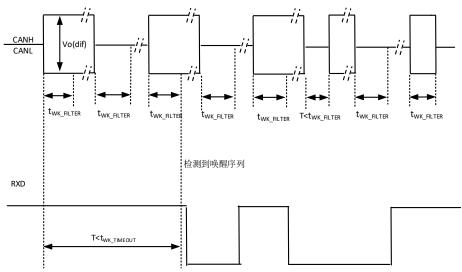
Figure 9-4 Wake-up Detection
