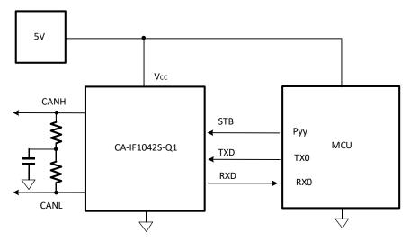
Figure 10-1 Typical Application Circuit for the CA-IF1042S-Q1
