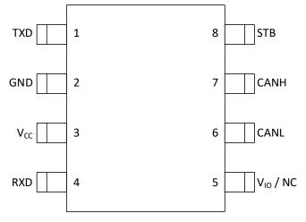
Figure 6-1 CA-IF1042x Pin Configuration
