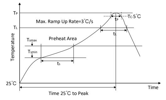
Figure 12- 1 Soldering Temperature (reflow) Profile
