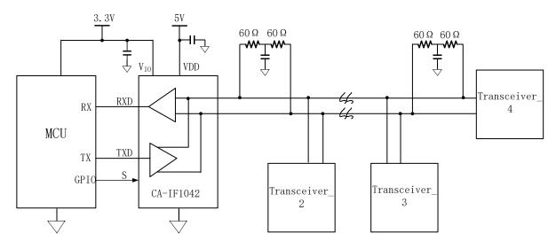
Figure 10-3 Typical CAN bus Network
