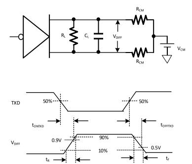
Figure 8-1 Transmitter Test Circuit and Timing Diagram
