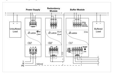
Fig. 4.4 General signals wiring
