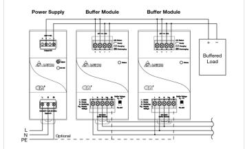
Fig. 4.3 Decoupling of buffered branches
