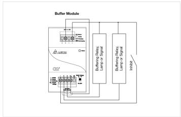
Fig. 4.5 Signals supplied from an external voltage
