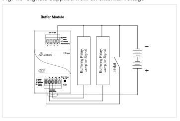
Fig. 4.6 Connection diagram with redundant operation
