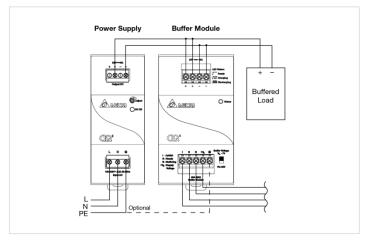
Fig. 4.2 Paralleling of buffer units
