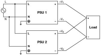
**Parallel Operation Connection Diagram** Fig. 4
