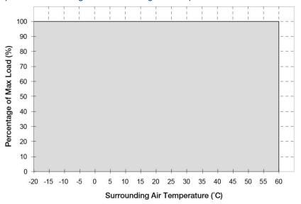
Fig. 2 No power de-rating across the entire operating temperature range  $(-20\,^{\circ}\text{C to }+60\,^{\circ}\text{C})$
