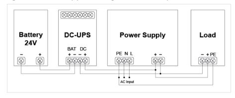
Fig. 4.2 Can be combined with redundancy module (DRR-40A)
