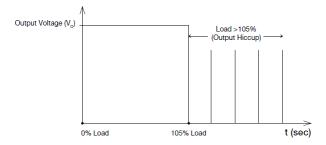
Additionally, if the  $I_0$  is <105% but >100% for a prolong period of time (depending on the load), the Over Temperature Protection (OTP) will be activated due to high temperature on critical components. The power supply will then go into latch mode until the fault is removed and the mains is reapplied.
