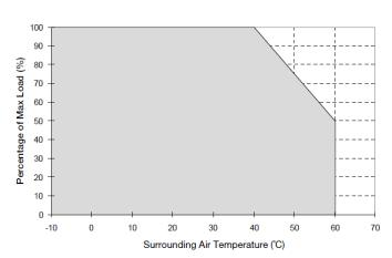
Fig.1.2 De-rating for Mounting Orientation A to F > 40°C de-rate power by 2.5% / °C
