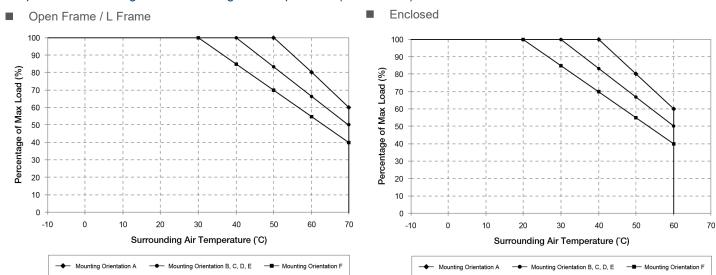
Fig.1.1 De-rating for Mounting Orientation A
