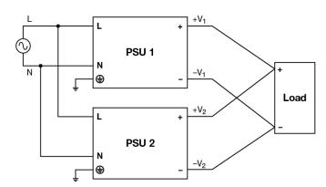
Fig. 4 Parallel Operation Connection Diagram
