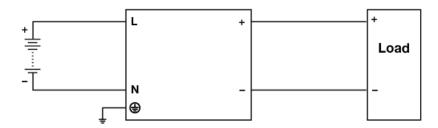
Fig. 5 DC Input Operation Connection Diagram
