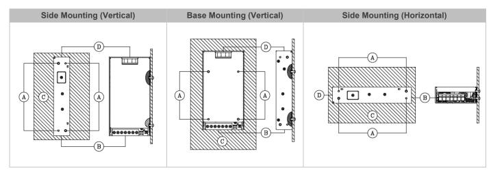
Fig. 2 Mounting Orientation
